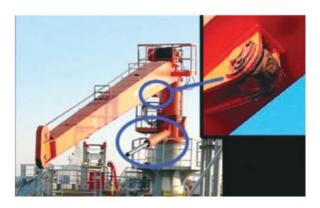
The company investigation found that the hydraulic cylinder eye attachment fitting had not been properly maintained. The <u>fitting was situated in a relatively</u> <u>inaccessible part</u> of the crane and <u>greasing of this part</u> had been neglected.
