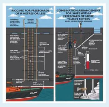
IMO RESOLUTION A. 1045/27 specifies requirements for the spacing of steps, location of spreader, clear of possible discharge, each step rest firmly on ship side, distance between each step, the rope diameter to use etc. The following factors shall be taken for maintenance and use of pilot ladder:
