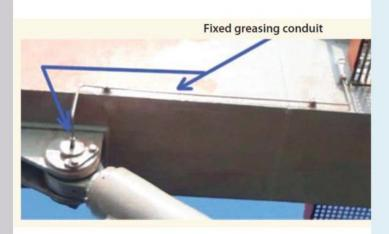
Additionally, the job card was updated. Instead of a generic maintenance description, the new card indicates specific greasing points to help crew to identify all maintenance areas. Finally, the manufacturer reviewed the design of cylinder eye bushings. Subsequent cranes will have bushings made of synthetic material instead of metal to reduce the risk of the steel pin seizing.
